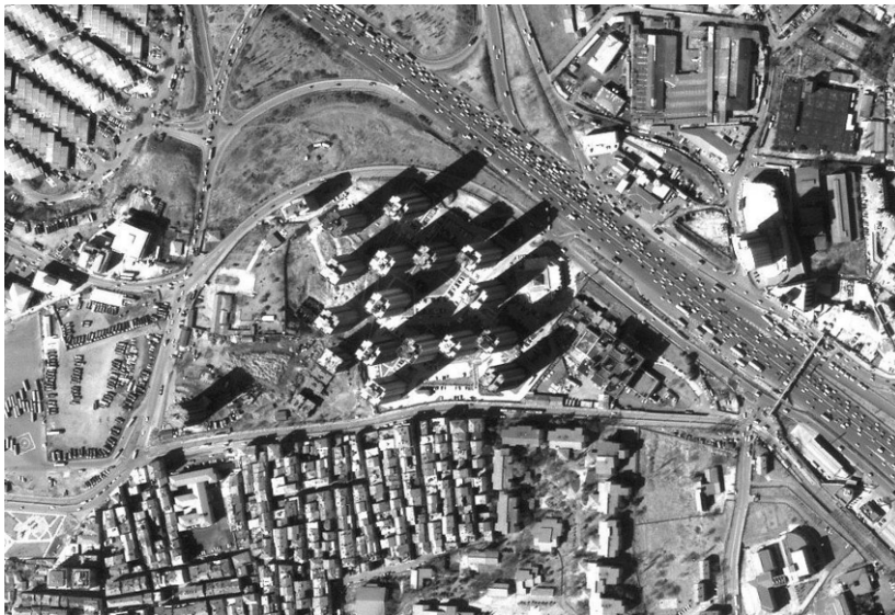
Figure 3. Subimage of ikonos A: high buildings leading to huge image displacement, long shadows and occluded areas.
